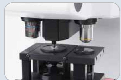
Unique Clemex self-level visor with built-in Test Block holder.
