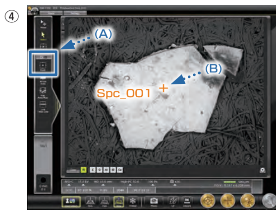
(A) Click the Point icon button. (B) Click a foreign material on the SEM image. These steps set the analysis positions.
