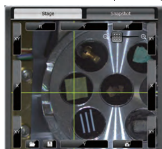
① Select a specimen area. In this image, plant leaves (biological specimen) is selected.
