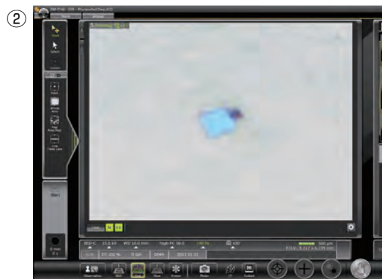
Magnify the CCD image*1 using Zeromag to confirm a foreign material.
