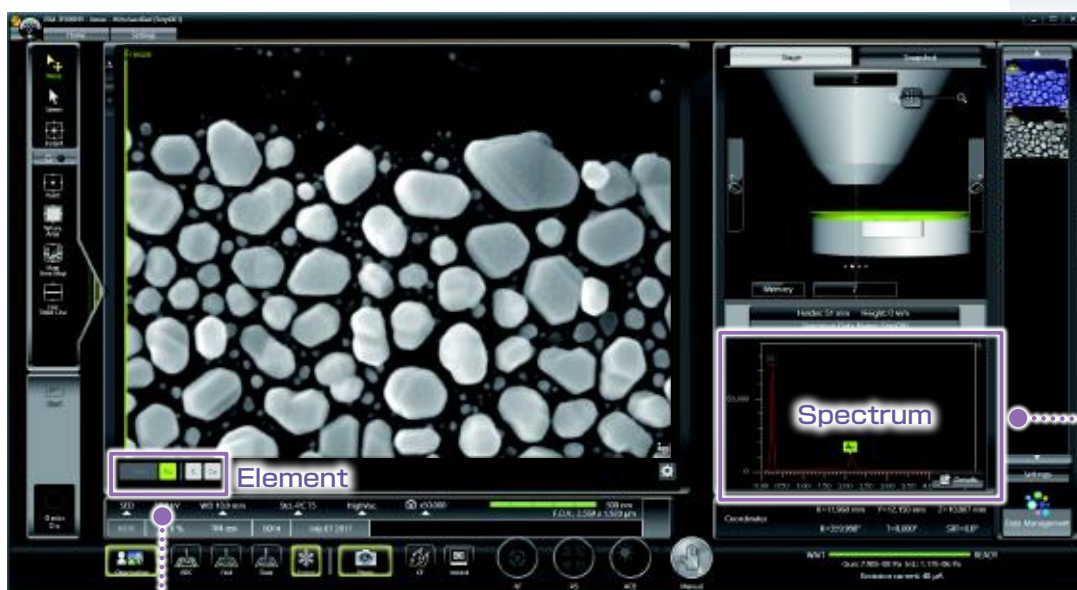
Specimen : Au particles on carbon, Accelerating voltage : 20 kV, Magnification : ×50,000 High-vacuum mode, Secondary electron image
