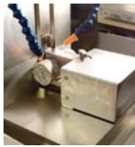
Pneumatic vice for core cutting on dual blade T260
