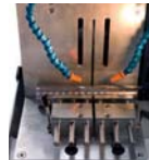
Left and right quick clamping vices Height 45mm Ref. 51210
