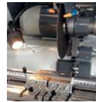
Left and right quick clamping vices Height 45mm Ref. 50906
