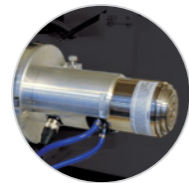
180 kV TRANSMISSION TARGET
