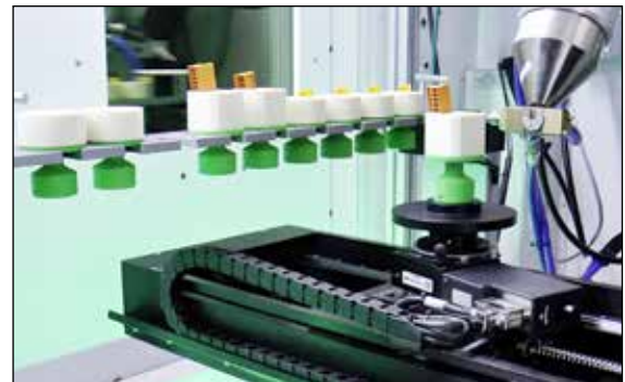
Semi-automated inspection allows automation of all tasks with multiple part loading.
