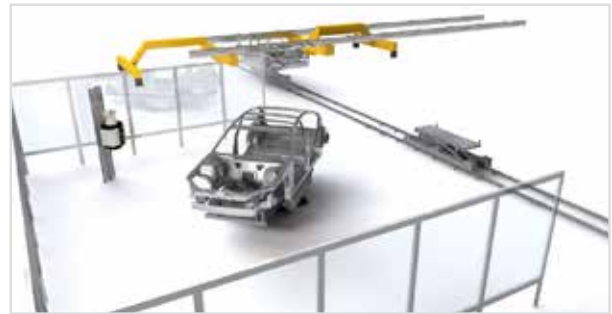
Line-side inspection with rotating table: A car body is taken from the line onto a rotating table. A Laser Radar on a fixed lift inspects the body from different sides.
