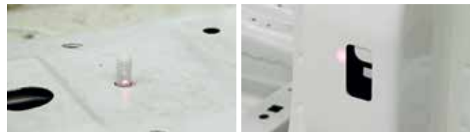
Features like holes, slots, pins, studs etc are inspected in an automated way at a scanning rate of 2000 points/sec
