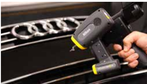
MMDx scanner is available in 50/100/200 mm stripe width
