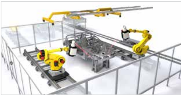
Line-side inspection: A car body is taken from the line and fully inspected. Two or four robots guarantee the highest inspection productivity. After inspection the body is re-inserted into the production line.
