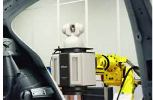
Laser Radar mounted on a robot is an innovative alternative for a traditional horizontal arm CMM
