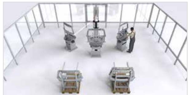
Component inspection: a single Laser Radar on a lift inspects front and back of multiple components on rotate tables.
