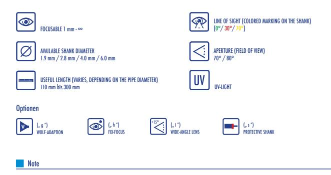
HIPP Borescopes Series FM have a standard aperture of 80 °. With a shank tube diameter of 1.9 mm, the aperture is 70 °. The option i = wide angle increases the aperture by 15 °. Matching protective shanks, according to the shank tube diameters, available.
