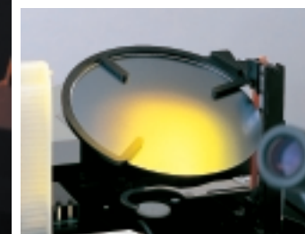
Back side center macro inspection (using a fiber optic illuminator)
