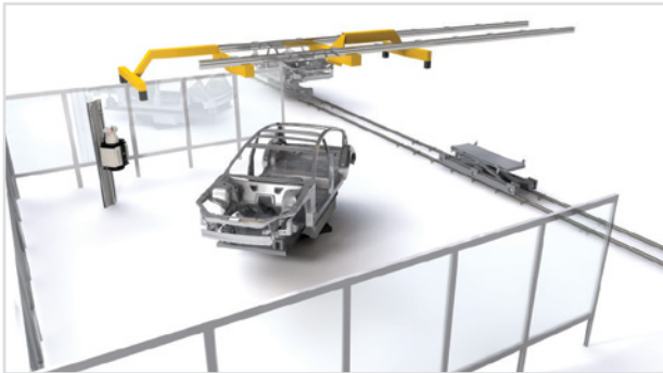
■ Line-side inspection with rotating table: A car body is taken from the line onto a rotating table. A Laser Radar on a fixed lift inspects the body from different sides.
