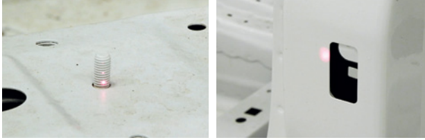
■ Features such as holes, slots, pins, studs can be quickly inspected using the Laser Radar
