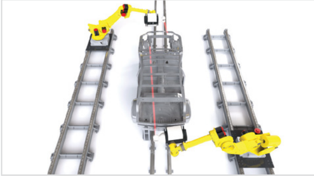
■ Inline car body inspection: On every car body, several features are inspected in the takt time of the line. After a series of passing cars, all critical features are measured.
