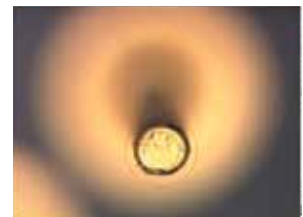
Circle probe appears on the abnormal pin location without measurement failure
