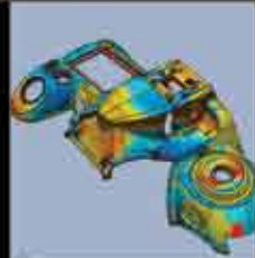
3D CAD Inspection - SLR Camera Cover
