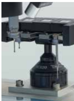
MCR20 Module Changing Rack Renishaw® is a registered trademark of Renishaw plc.
